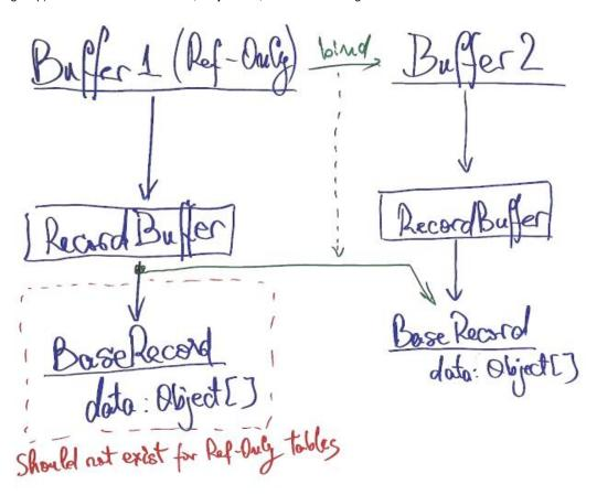
So we have the lowest level object, the data array of similar size and corresponding properties types (validated while binding). All we need to do is redirect R/W accesses of buffer1.currentRecord.data[i] to buffer2.currentRecord.data[i]. The Record/BaseRecord have to be kept since the access will still be done via the DMO interface, but the data it writes to/read from is temporarily (during bind) changed (maybe the lower green arrow should be moved even lower).
